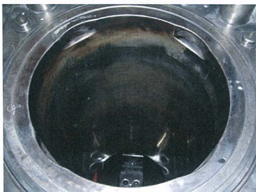
Corrsion and Scuffing on the surface of Cylinder
