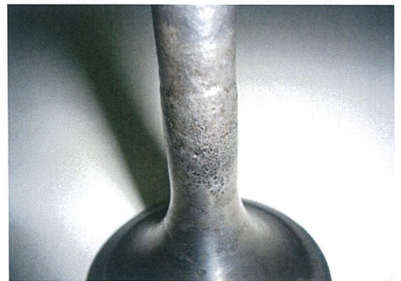
Corrosion of exhaust Valve Stem
